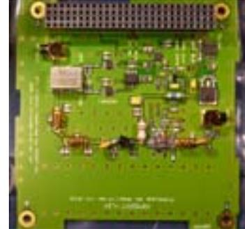
In addition to the RF amplifier, the PA board contains four sensors that gather data for the satellite's telemetry. The sensors are:
