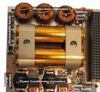
This type of supply is capable of providing power directly from the solar panels in the event that, after some time in space, the battery no longer holds its charge. This will permit sunlight-only operation of the spacecraft after a battery failure; this was an early mission requirement.
